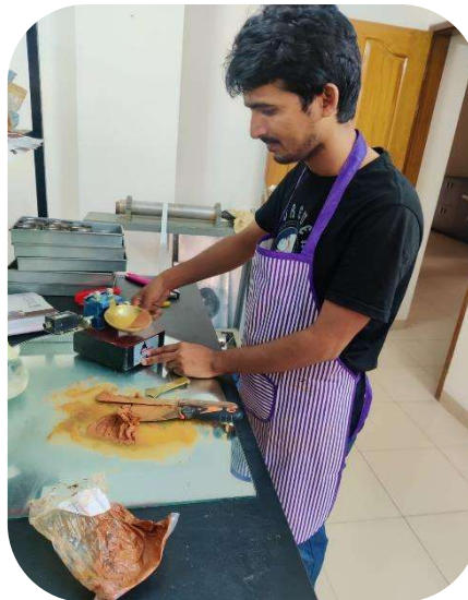
Performing Atterberg Limit Test
