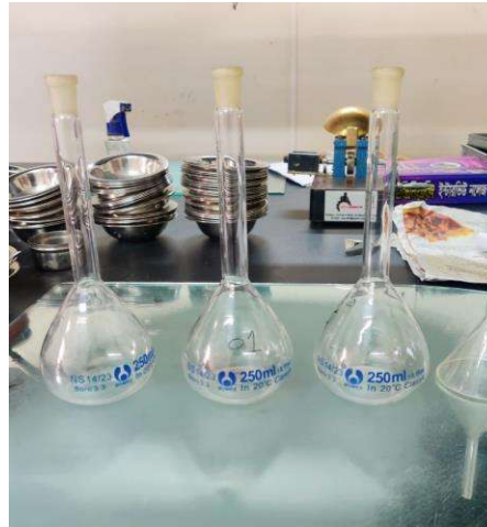
Pycnometer used in Specific Gravity Determination
